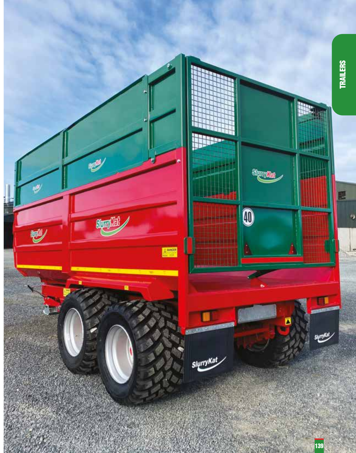
14T/18ft Panterra Silage Trailer c/w 560/60 floatation tyres & semi auto silage door
