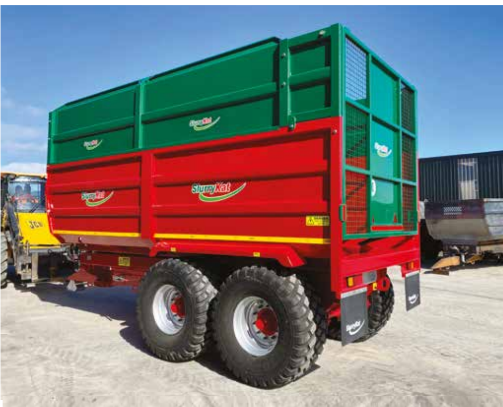
14T/18ft Panterra Silage Trailer c/w 560/60 floatation tyres & semi auto silage door
