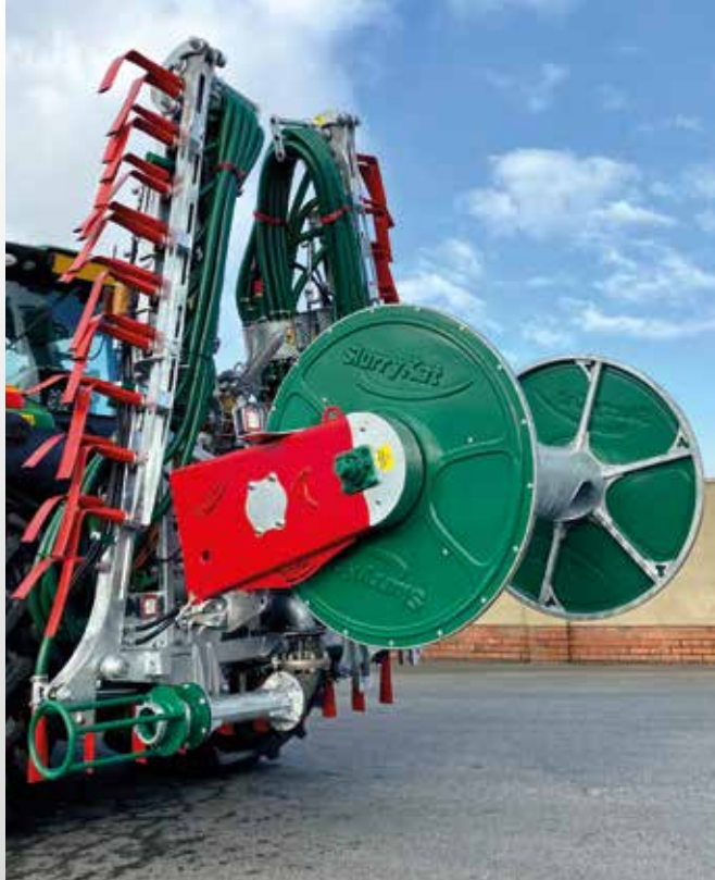
800m reelers front & rear – 1600 metre hose capacity
