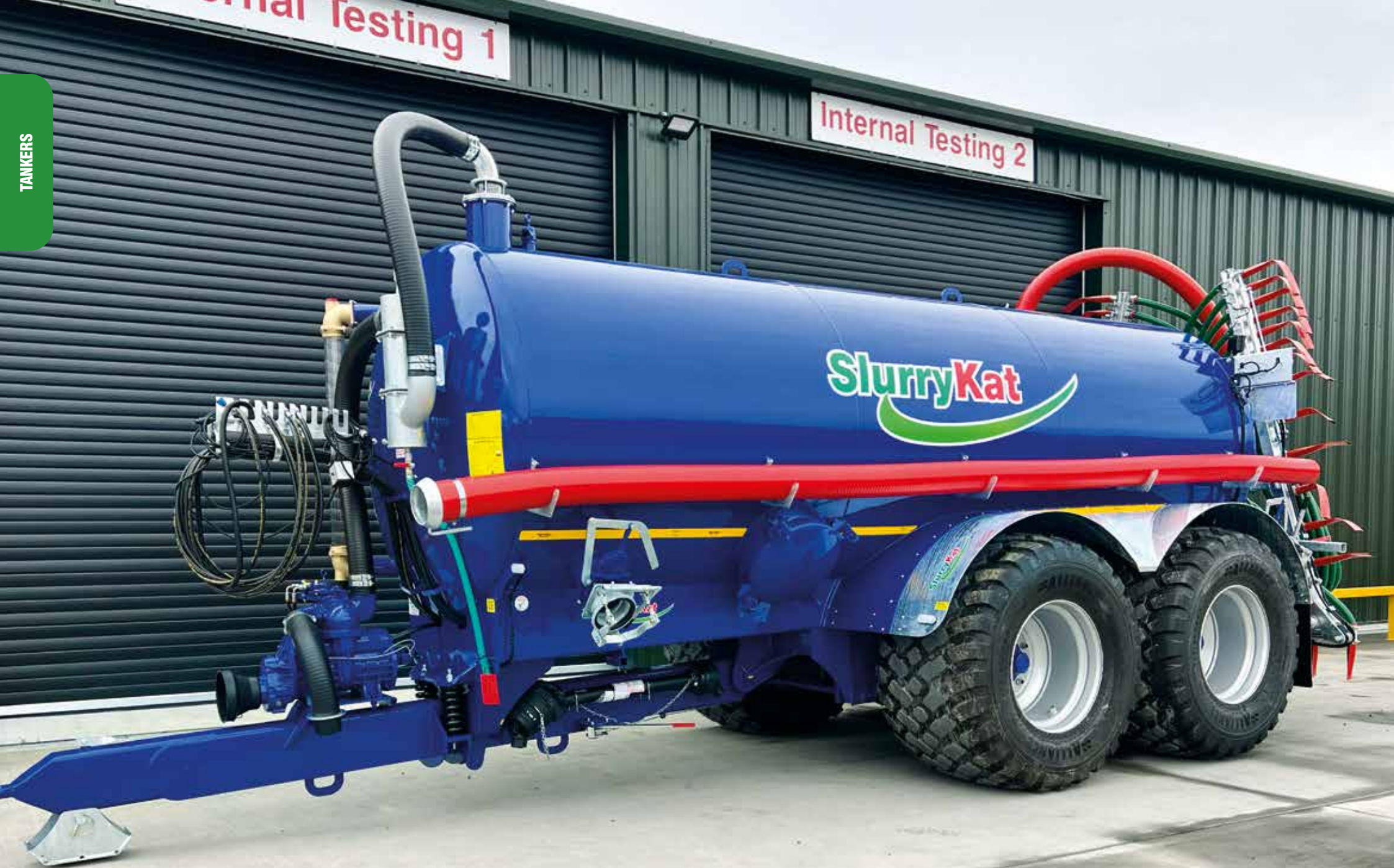
3500G/16m 3 Premium Plus Tanker, 710/R26.5 tyres, 9m Farline dribble bar
