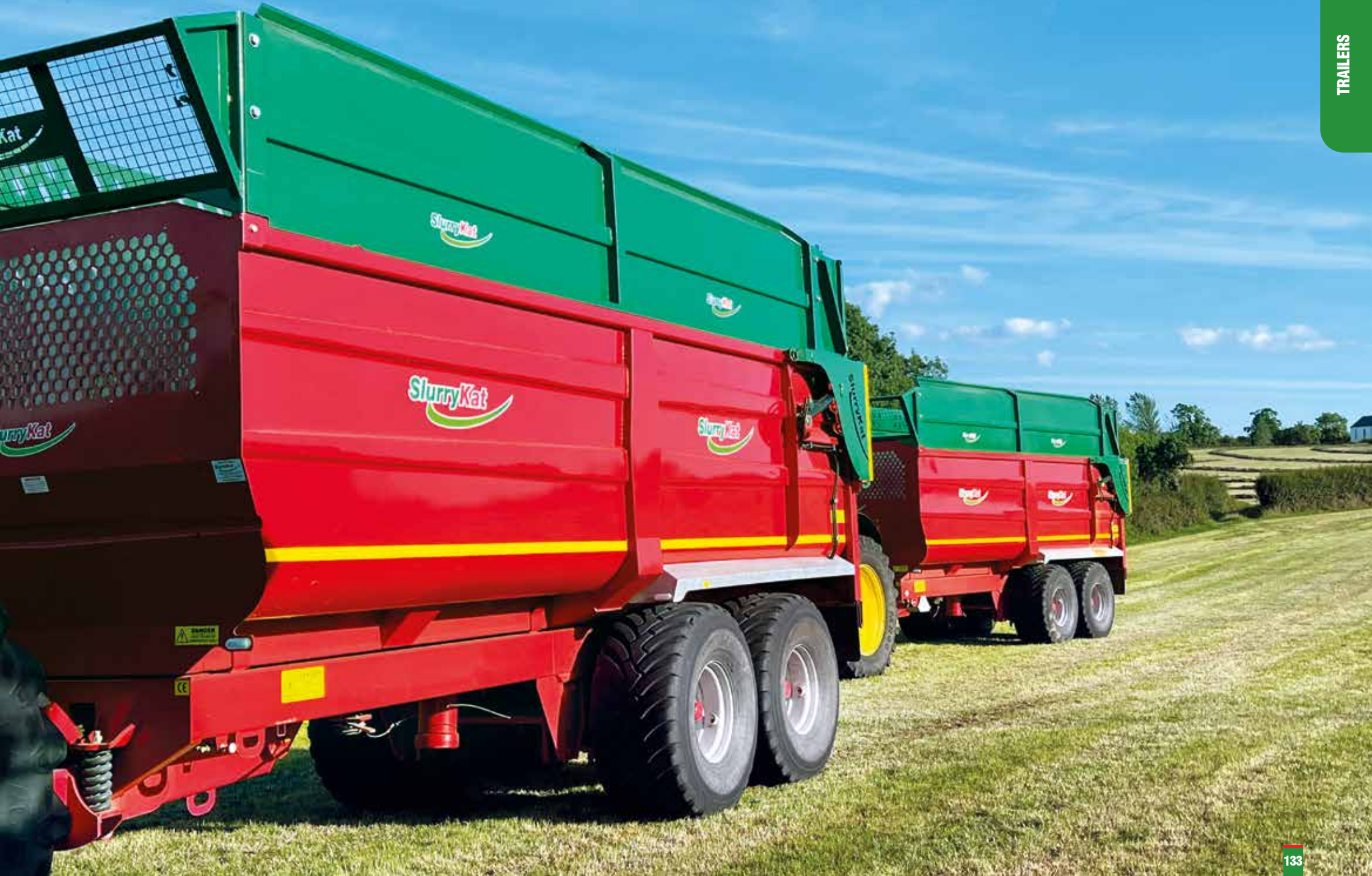
22ft ProLine silage trailers, 580/65R22.5 Flotation tyres
